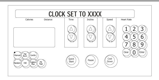
This test allows the user to see the current time set on the frame tag real time clock. If the communication is bad or the frame tag is unplugged the following messages will appear. Refer to the troubleshooting section for corrective action.
